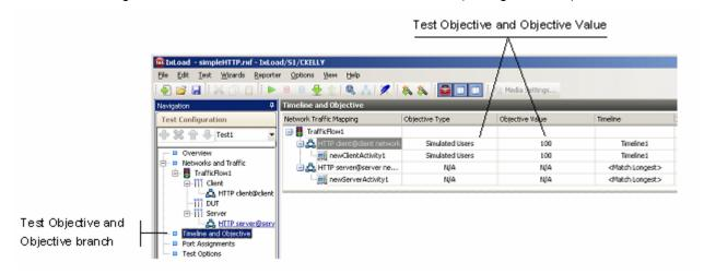
The windows on this branch display the timeline (the timing of events that occur during the test, such as when the simulated users and HTTP server are brought online) and the Test Objective.
