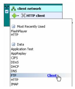
IxLoad adds a new FTP Client activity to the HTTP client (as shown below).
