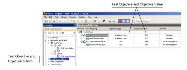
The windows on this branch display the timeline (the timing of events that occur during the test, such as when the simulated users and HTTP server are brought online) and the Test Objective.
