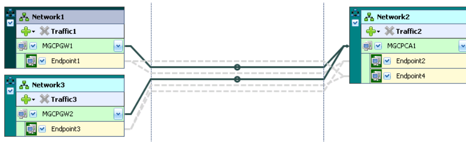
Figure 5-88. Two GWs with Controlling CA
