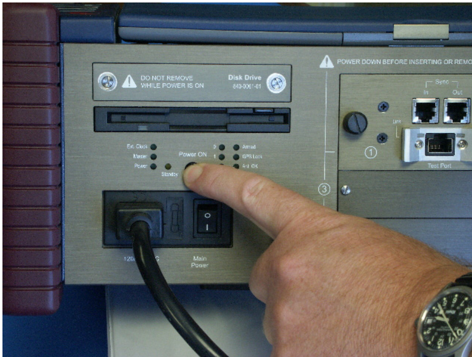
Figure 11-8. IXIA 250 Standby Switch
