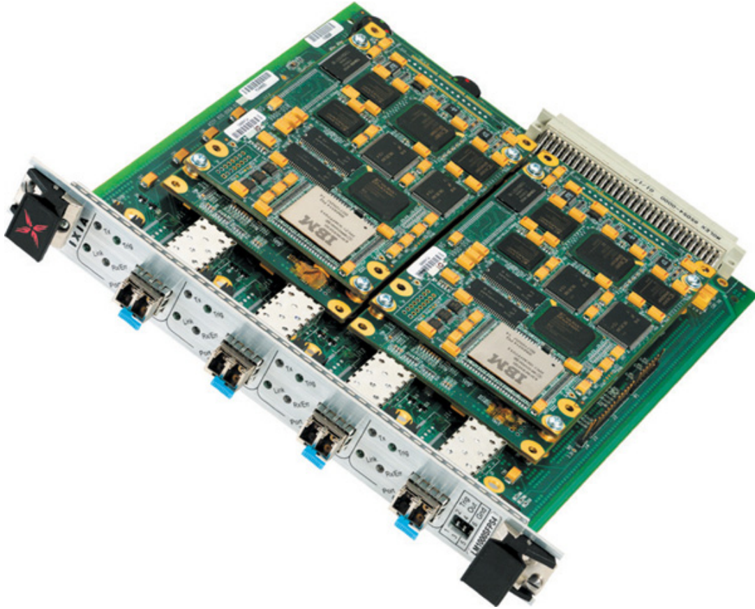
Figure 25-1. LM1000SFPS4 Load Module
