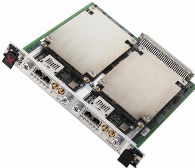
Figure 22-1. LM622MR Load Module with Pluggable PHYs Installed
