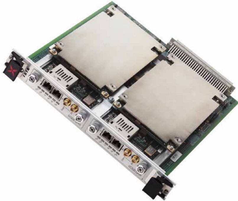
Figure 26-1. LM622MR Load Module with Pluggable PHYs Installed
