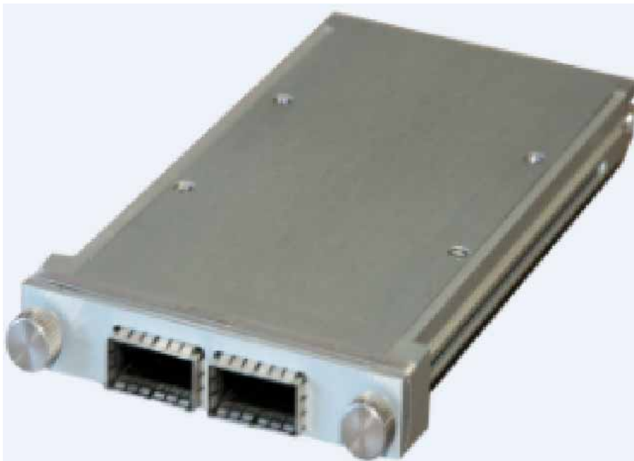
Figure 15-3. CFP-to-QSFP+ Dual-Port Interface adapter
