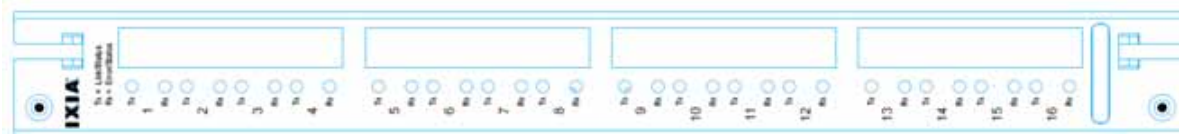
Figure 33-5. Front panel of FlexAP10G16S/FlexFE10G16S
