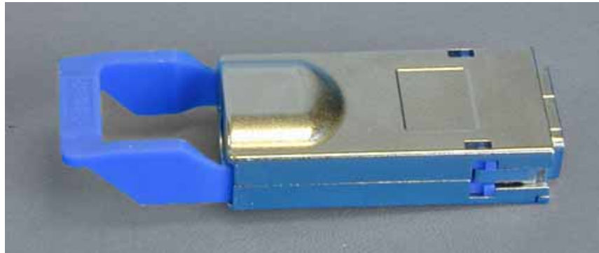
Figure A-3. XAUI Front Panel Loopback Connector
