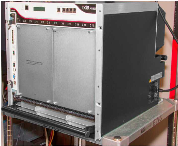
Figure: XGS12 Mounted on Rack
