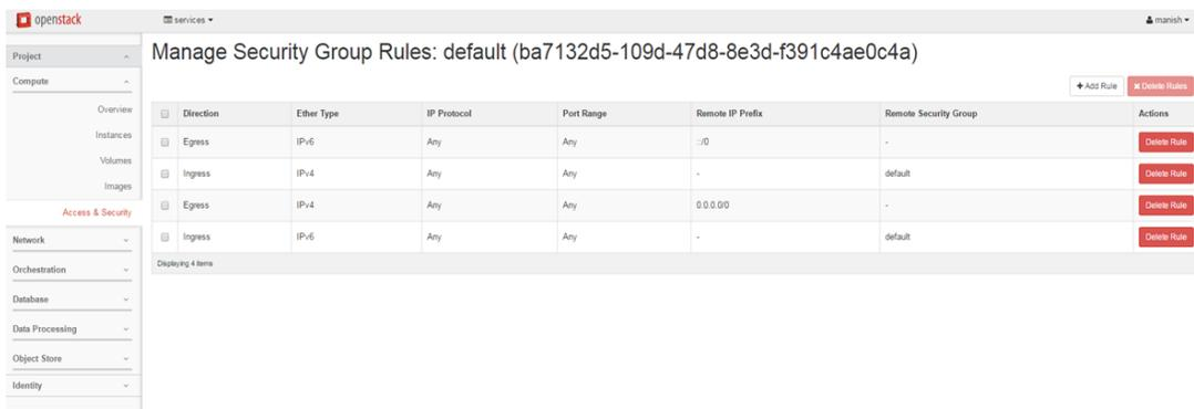
The screenshot shows the 'Manage Security Group Rules' page for the 'default' group. The page title is 'Manage Security Group Rules: default (ba7132d5-109d-47d8-8e3d-f391c4ae0c4a)'. It features a table with columns: Direction, Ether Type, IP Protocol, Port Range, Remote IP Prefix, Remote Security Group, and Actions. There are four rules listed, each with a 'Delete Rule' button.
