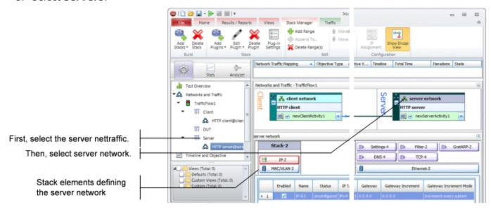
As with the client network, the tabs to the right display the network parameters that define the server network. The figure below shows how the network controls correspond to the test topology.
