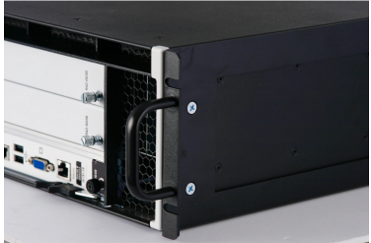
Rack Mounts attached to the front of the chassis
