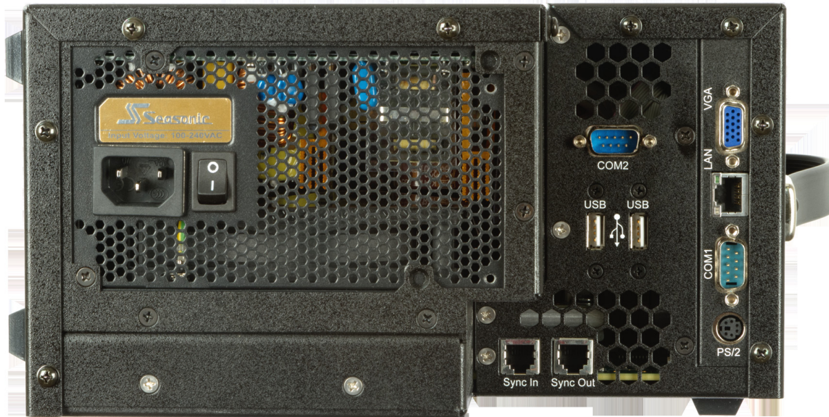
Figure 12-2. Ixia 400T v2 Chassis - Rear View
