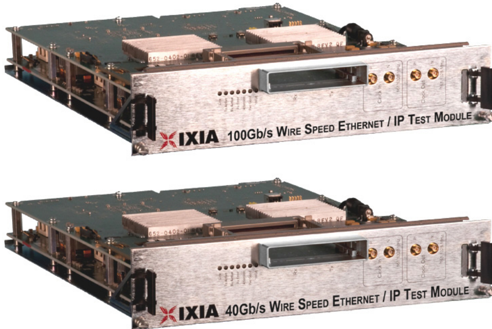
Figure 24-2. 40GE LSM XMV QSFP Load Module
