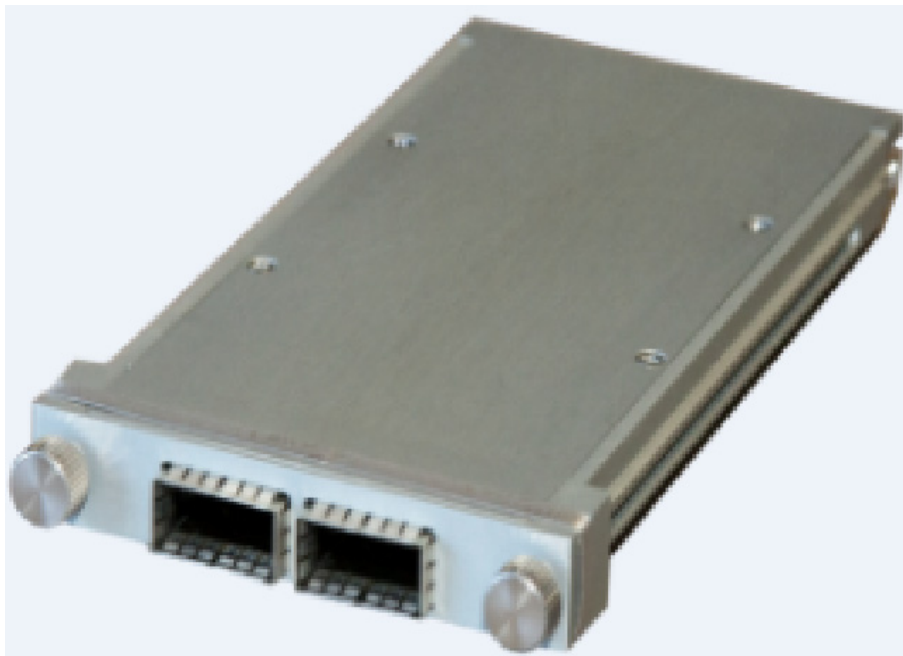
Figure 16-3. CFP-to-QSFP+ Dual-Port Interface adapter
