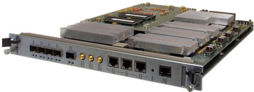
Each XAir board supports one sector, with 1 Gbps Ethernet ports connected to the IxLoad Xcellon NP or IxCatapult m500/p250 chassis. It also supports up to 4 CPRI interfaces to an eNB or to Ixia's Remote Radio Head r10 units that cover all FDD & TDD frequency bands.
