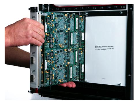
3. Gently slide the load module into the slot by pushing on the front of the load module.
