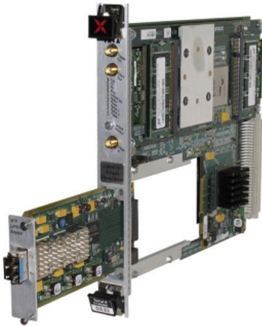
Figure: XFP-ADAP-02 Carrier Card
