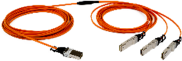
Figure: 100GE CXP-to-3x40GE QSFP+ AOC fiber fan-out cable
