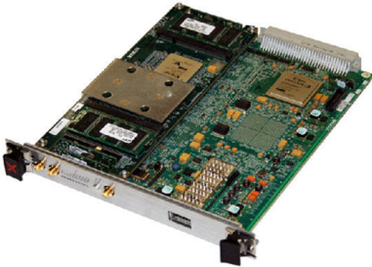
Figure: LSM10GMS-01(MACsec Carrier Card)
