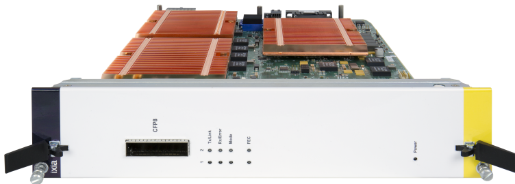
Figure: K400 Module-CFP8-400GE
