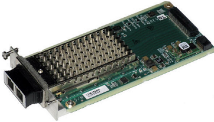
Figure: XFP-ADAP-02 Carrier Card
