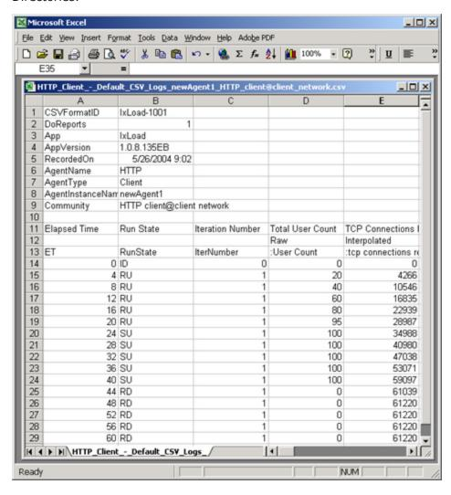
Each time you run a test, IxLoad creates a new directory to store the CSV and log files in; it names the directory based on the repository name, test configuration, date and time of the test, and the activity model and network group used. For example, the format for the client-side file is:
