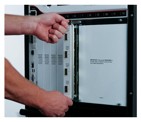
3. Grip the front of the load module and pull it out of the chassis. When the load module is partially out, support the bottom of the load module.
