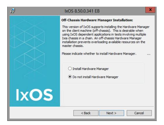
As described in the dialog box, it is advisable to install the Hardware Manager off-chassis for applications that run tests over chassis chains.
