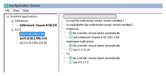
For example, Application Selector indicates that, for IxOS version 8.40.1400.5, the compatible version IxNetwork 8.50.1501.4, is installed. It also indicates the default No override selection for the Tcl version.
