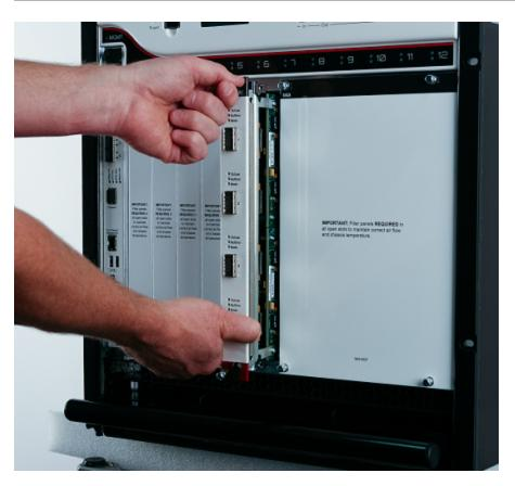
4. Place the load module into an ESD bag or container, to prevent damage while handling or transporting it.
