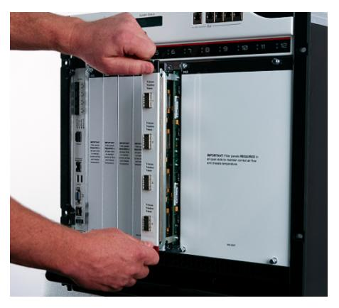
2. Gently grip the ejectors and pull the load module a short way—about 1 inch (3 cm)—out of the chassis.
