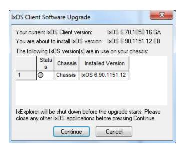
The **IxOS Client Software Upgrade** dialog box displays the current version of the client computer software and the server computer software. Select **Continue** to begin upgrading the client computer software.
